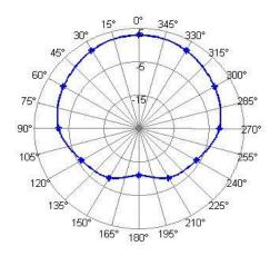
Azimuthal power pattern. DBi values when Internally Mounted at 915MHz
