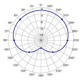
UBM-S1 Measurements at 700MHz
