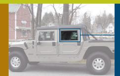
Fractal antenna technology, implemented in transparent conductive film, makes covert capability possible with a mission-capable antenna system that operates over a huge frequency range.
