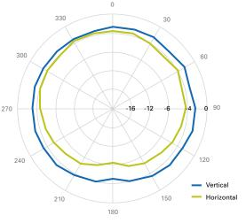
\*Readtenna™ 900 has excellent azimuthal pattern and average gain of -2dB relative to a dipole. Note that an ideal circularly polarized antenna is -3dB relative to a dipole.
