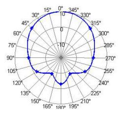
Typical Azimuth DBi Values on drywall for FDY Versions:
